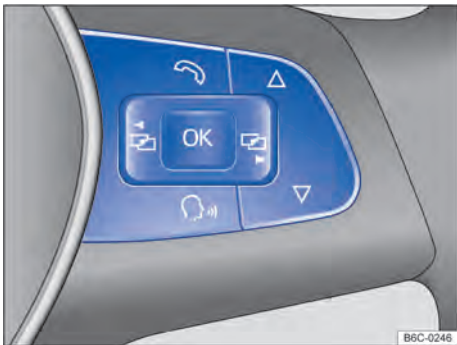
Fig. 20 Right hand side of the multifunction steering wheel: menu operation and instrument cluster information exhibit buttons.
