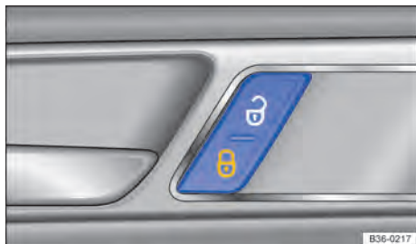
Fig. 56 On the driver door: central locking button.
