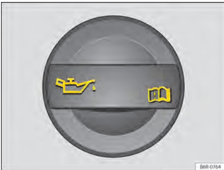
Fig. 186 On the engine compartment: engine oil opening lid.
