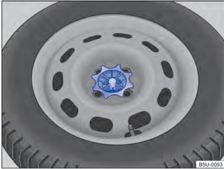
Fig. 196 On the luggage compartment: spare wheel fastening handwheel.
