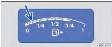
Fig. 13 In the analogue instrument cluster: fuel gauge.
