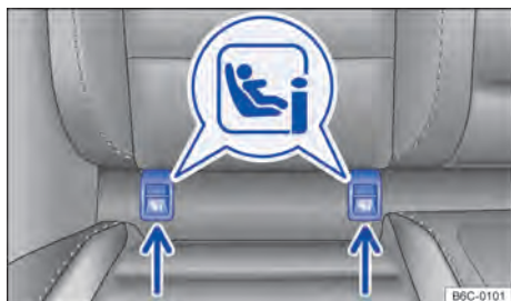
Fig. 44 On the vehicle seat: identification of lower retaining rings for child seats.
