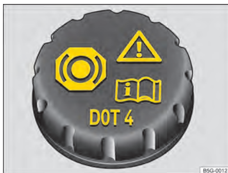
Fig. 189 On the engine compartment: brake fluid reservoir cap.
