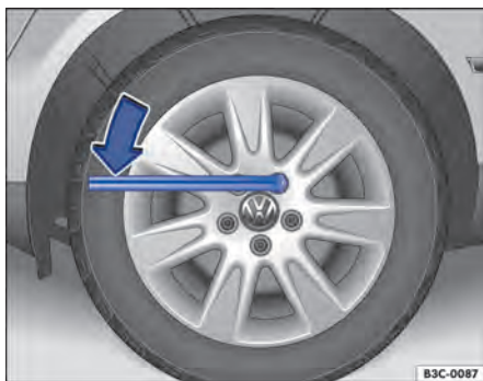
Fig. 200 Changing the wheel: loosen wheel bolts.
