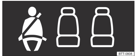
Fig. 25 Seat belt status indicator for rear seats in the instrument cluster display.
