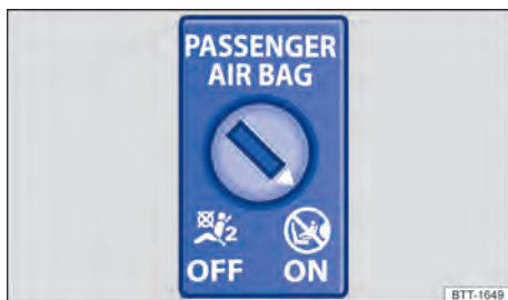
Fig. 39 On the dash panel on the front passenger side: key activated switch to enable or disable the front passenger front airbag.
