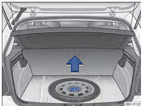
Fig. 159 On the luggage compartment, under the floor lining: spare wheel and vehicle toolkit.
