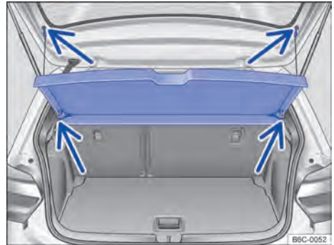
Fig. 151 In the luggage compartment: remove and install the luggage compartment cover.
