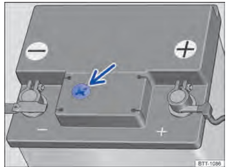
Fig. 190 On the engine compartment: example of display position on the upper side of the vehicle battery.
