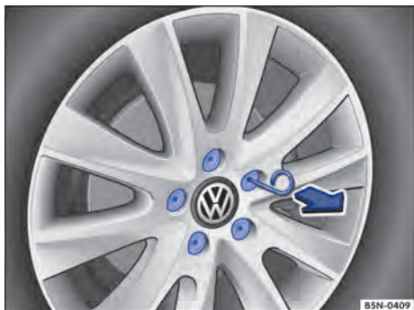
Fig. 199 Removing the wheel bolt caps.
