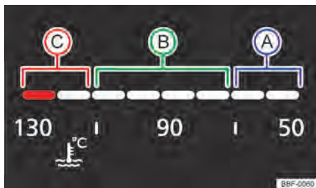
Fig. 16 Engine coolant temperature indicator in the digital instrument cluster (version 2): (A) cold zone; (B) normal zone; (C) warning zone.
