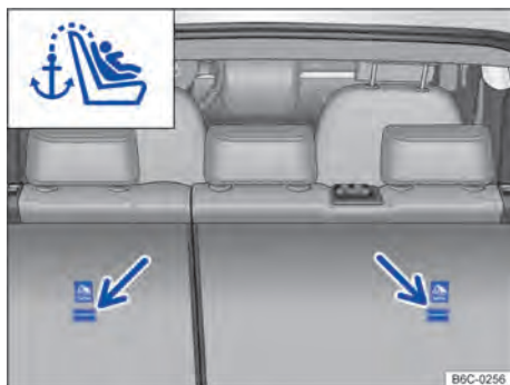
Fig. 45 retention eyes for the top tether on the back side of the rear seat.
