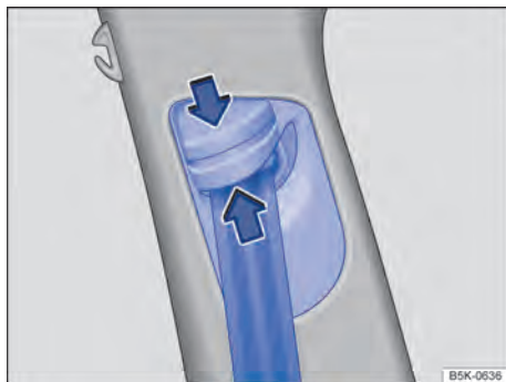
Fig. 35 Next to the front seats: seat belt height adjuster.
