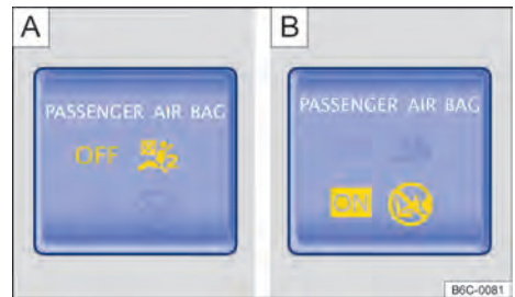
Fig. 36 In the upper part of the centre console: front passenger front airbag indicator lamp off [A] or on [B].
