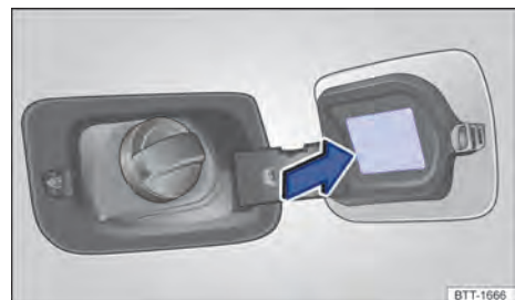
Fig. 194 On the inner side of the fuel tank flap: tyre pressure label.
