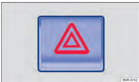
Fig. 49 On the upper portion of the centre console: warning lamp switch.
