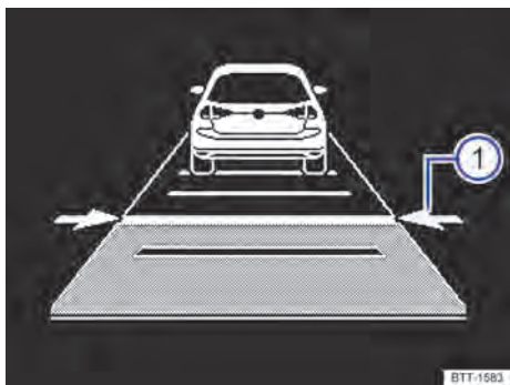
Fig. 102 On the instrument cluster display: adjust the distance (schematic view, the ACC will adjust).
