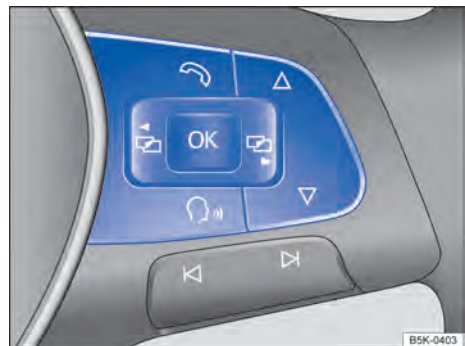
Fig. 18 Right hand side of the multifunction steering wheel: menu operation and instrument cluster information exhibit buttons.
