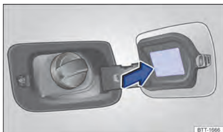
Fig. 192 On the inner side of the fuel tank flap: tyre pressure label.
