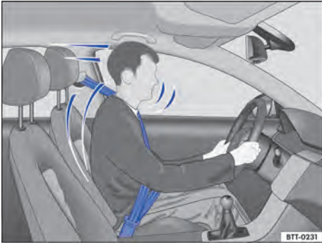
Fig. 28 Driver restrained by a properly positioned seat belt during a sudden braking manoeuvre.
