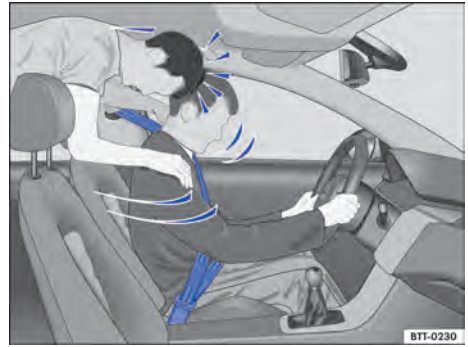
Fig. 27 The unbelted rear passenger is thrown forward violently, hitting the belted driver.
