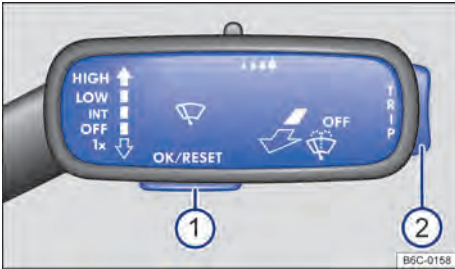
Fig. 17 Vehicles without multifunction steering wheel: press button ① on the windscreen wiper lever to confirm the menu items and rocker switch ② to switch between menus.
