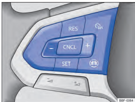
Fig. 97 Left side of the multifunction steering wheel (version 2): speed limiter operating buttons.
