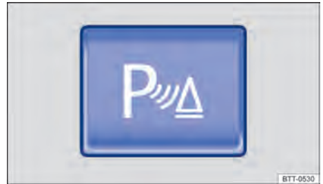
Fig. 104 On the centre console or on the radio display: button for turning the parking aid on and off.
