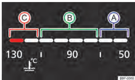
Fig. 14 Engine coolant temperature indicator in the digital instrument cluster (version 2): (A) cold zone; (B) normal zone; (C) warning zone.
