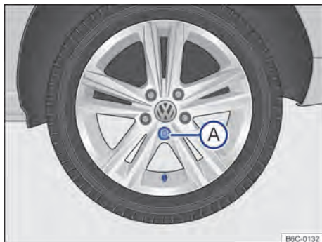
Fig. 202 Wheel replacement: wheel bolt removal sequence.
