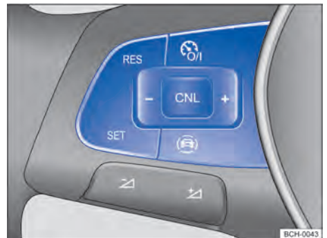
Fig. 96 Left side of the multifunction steering wheel (version 1): speed limiter operating buttons.
