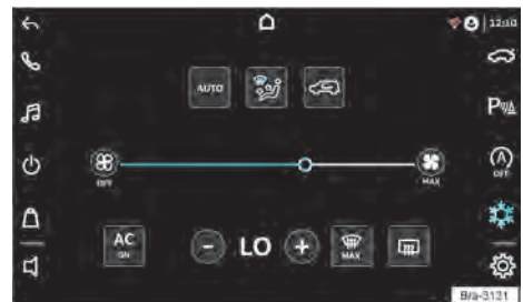
Fig. 145 Air conditioning in multimedia.
