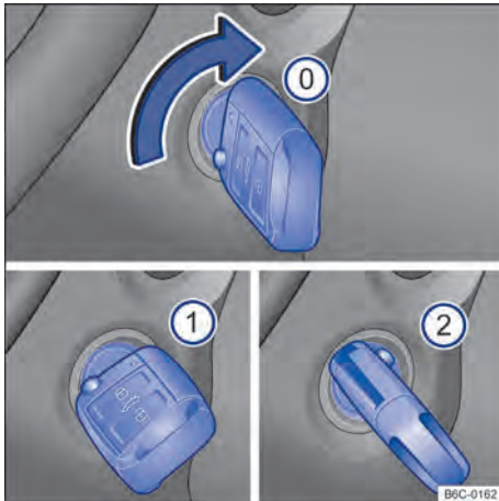
Fig. 87 Next to the steering wheel, to the right: vehicle key positions on the ignition cylinder.
