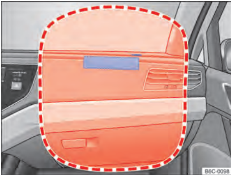
Fig. 36 Installation location and expansion zone of the passenger front airbag.
