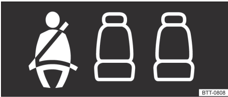
Fig. 23 Seat belt status indicator for rear seats in the instrument cluster display.
