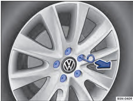
Fig. 197 Removing the wheel bolt caps.
