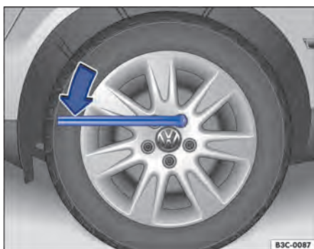
Fig. 198 Changing the wheel: loosen wheel bolts.
